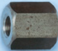
(1031 RN) inside thread G 3/8" to inside thread M 14 x 1.5, fits between packer (1031), nipple (1031N)
