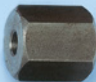
(1025 RN) for high pressure inside thread G 1/4" to inside thread M 10 x 1.0, fits between packer (1025), nipple (1025N)
