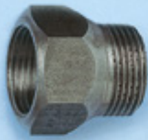
(1039 R) inside and outside threads G 3/4" to inside thread M 14 x 1.5, fits between packer (1039), nipple (1031N), stop cock (1175) and (1185)
