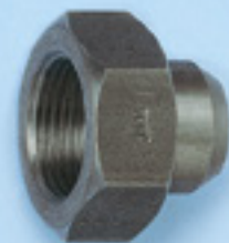
(1039 R) inside and outside threads G 3/4" to inside thread M 14 x 1.5, fits between packer (1039), nipple (1031N), stop cock (1175) and (1185)
