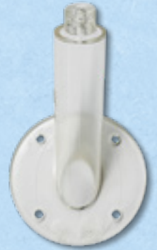
Adhesion packer round (1135A)< made of transparent polycarbonate, with bevelled filler neck, outside thread M 10 x 1.0 weight circa 8 g
